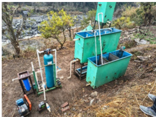
Prototype of Decentralized Wastewater Treatment Unit installed at the Project site (Nandli, Mandi, Himachal Pradesh)
