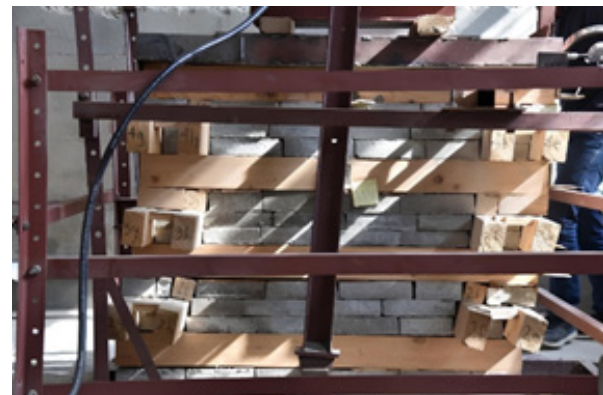
Testing of scaled-down traditional kath-kunni wall on the proposed reaction frame
