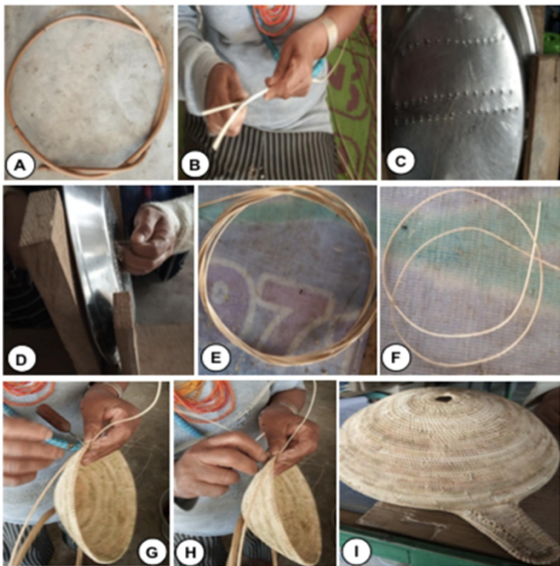
PLATE - II: A. Dried oso ( Calamus spp.); B. splitting of Oso with help of Dao ; C & D. conversion of splitted oso into pyalo ; E. Pyalo ; F- Somo ; G & H. weaving of somo over pyalo using silo ; I. Main frame.
