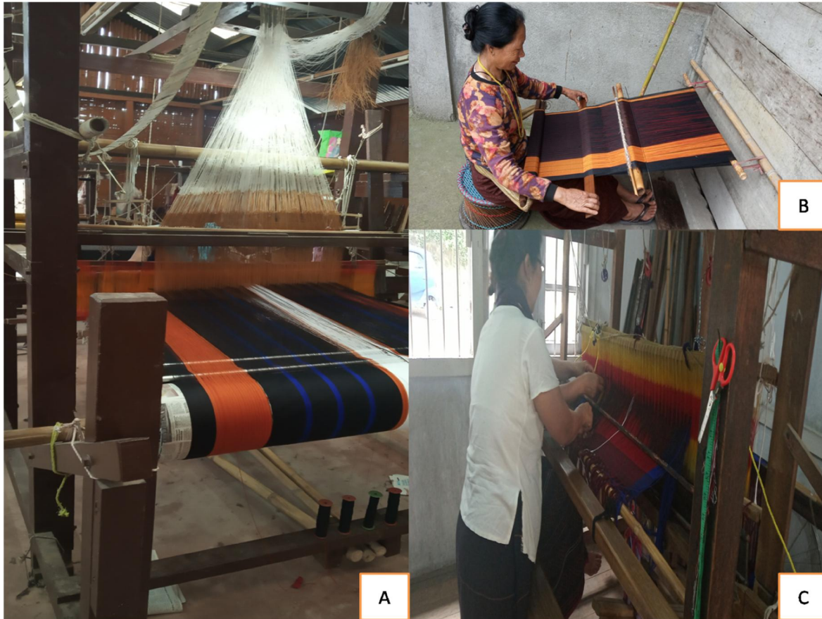
Fig. 2: A- Jacquard loom; B- Loin loom (Chichin); C- Flying shuttle loom
