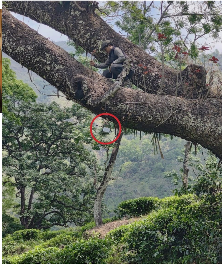
SM4BAT FS placed on a tree to record echolocation call of free-flying bats - Deoashis Thapa
