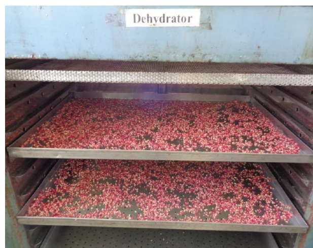
Mechanical cabinet drier
