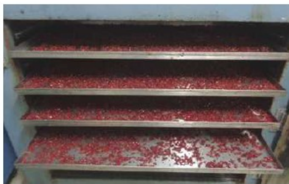
Mechanical cabinet drying
