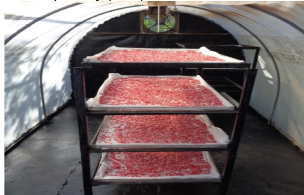
Solar tunnel drier
