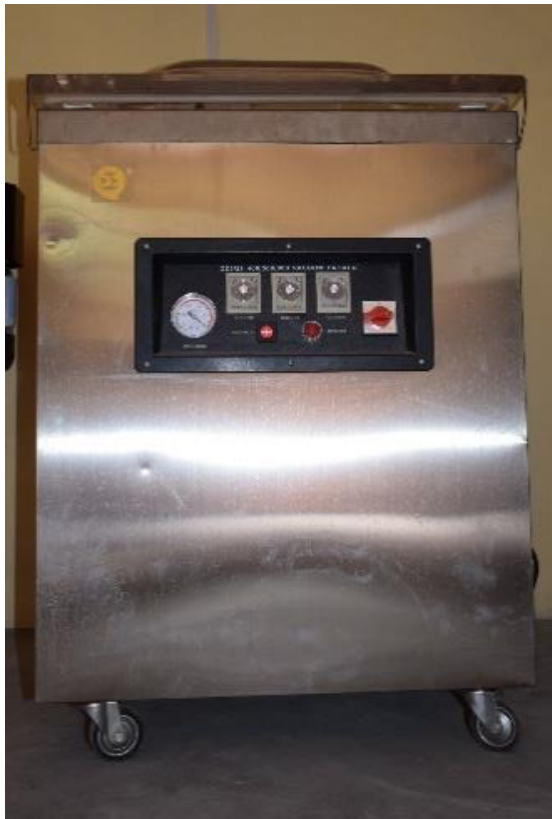
Fig. 44 Vacuum ppackaging machine
