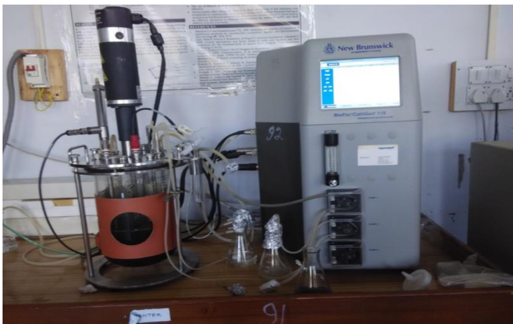
Fig Bioconversion process in a stirred tank bioreactor
