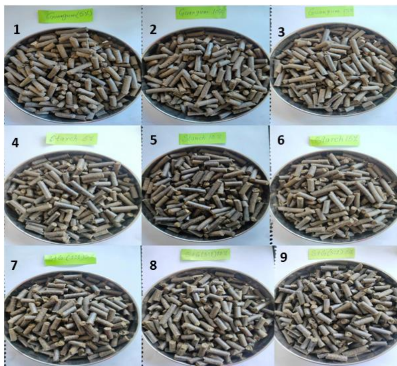
Figure 9. Biomass samples of different binder concentrations (1) 5% of guar gum, (2) 10% of guar gum, (3) 15% of guar gum, (4) 5% of starch, (5) 10% of starch, (6) 15% of starch, (7) 5% of starch and guar gum (1:1 ratio), (8) 10% starch and guar gum (3:1 ratio), and (9)15% of starch and guar gum (5:1 ratio).
