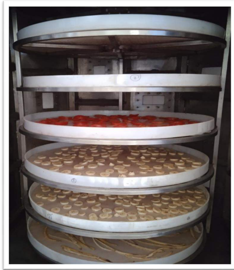
Figure 1: Trays containing raw material for drying in a vacuum assisted microwave drying
