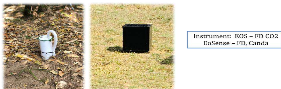
Fig.4 Soil CO 2 efflux installed at Oak and Pine site.
