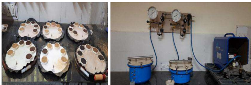
Fig. 4. Laboratory pressure plate soil moisture experiment set-up: (left) Saturated soil samples placed on the ceramic pressure plates; (right) Pressure plate apparatus consisting of two pressure vessels, two pressure measurement unit, and pressure generator.
