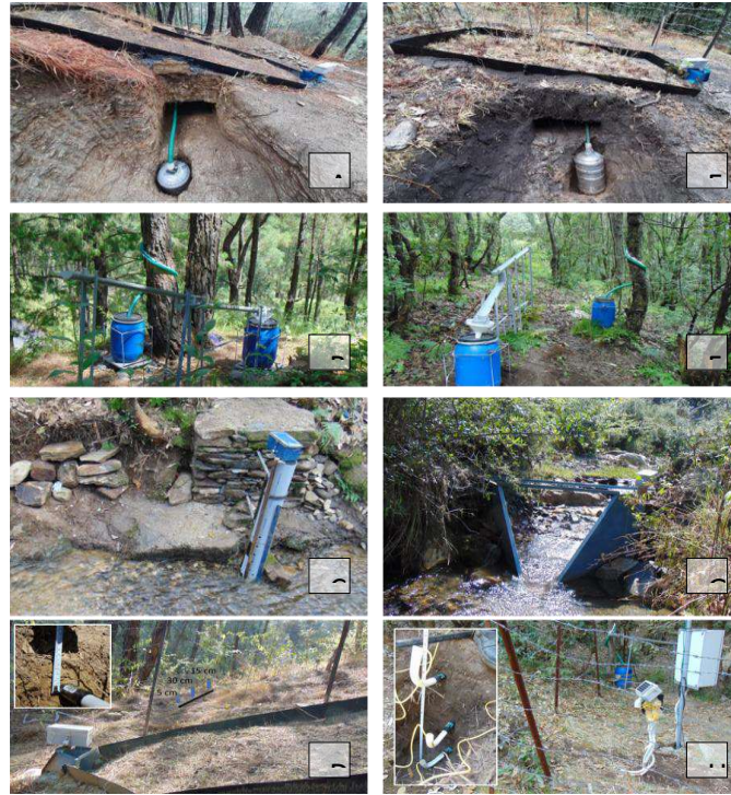
Fig. 3. Photographs of field installations at Pine site (A, B, C, D) and Oak site (E, F, G, H); A & D are surface runoff plots with a view of the collection system for soil leachate; B & E are stem flow and throughfall collection systems; C is the stilling well at the outlet of Sitlakh watershed while F is the 3 feet flume at the outlet of Papoli watershed; D & H are installation pictures of soil moisture sensors.
