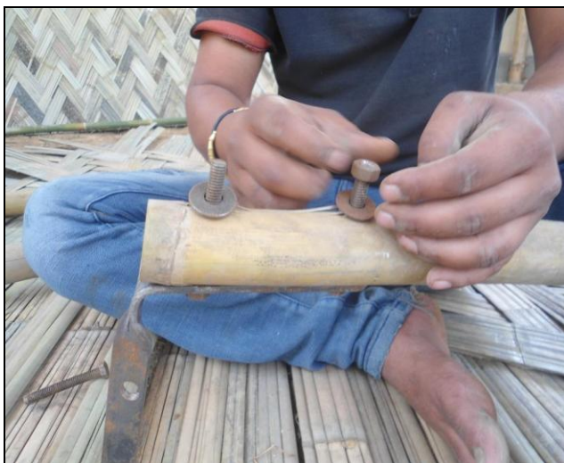
4: Fastening the clamp with the bamboo
