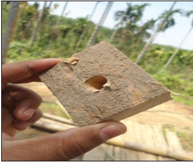
A section of bamboo can be used in case a bolt length go excess
