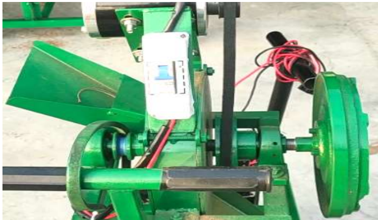
Fig.4 Switch is provided to turn on the motor in crusher
