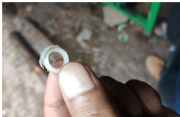
c) Damaged washer removed and replaced
